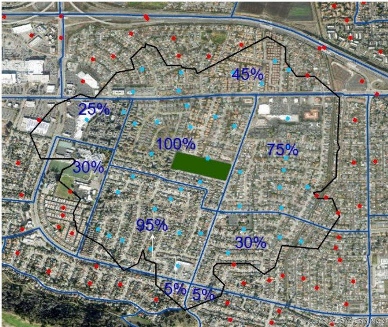
Figure 3 – To calculate populations using aerial apportionment, the population of each demographic for each block group is adjusted by the percentage of the block group’s areas (blue numbers) inside the summary area (the black service area in this case) and then the adjusted percentages are added to produce a population number. As the leftmost block group shows, this method does not consider the population distribution and can lead to less accurate results.
