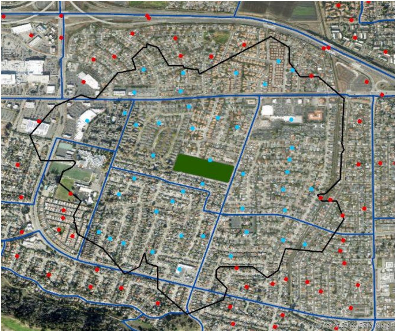
Figure 2 - Visualization of the block point method using the same park shown in Figure 1. Each block group (dark blue lines) contains multiple block points (red and blue points). Each block point represents a fraction of the population of the block group it resides in. The population of each block point for each demographic can be calculated using this fraction. To calculate the population served in a given region (in this case, the service area shown in black), the demographic populations for all points within the region (blue points) are summed. Although nine block groups intersect the service area, only six contain block points within the service area. The block point method takes variations of population density within a block group into account.
